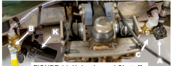
FIGURE 14, Unloader and Shutoff
