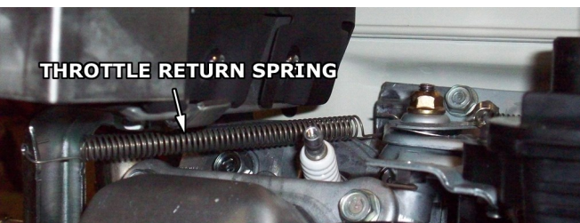
FIGURE 22 , Adjusting engine speed
