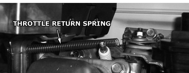
FIGURE 22 , Adjusting engine speed
