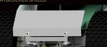
The stainless steel spray shield blocks spray drift that would normally attract fertilizer onto the hood, eventually clumping off and creating brown spots
