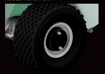
Wheel weights deliver extra traction, stability and cornering to compliment the tighter turning radius.
