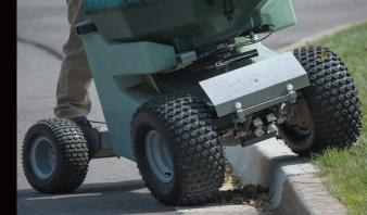
The patented articulating joint connecting the front half of the Triumph to the rear sulky provides tight turning, stability and shock absorption on rough ground.
