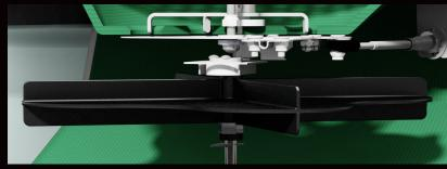
When one side of the impeller wears out, flip it over to expose a new platter...now that's smart
