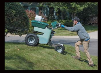
The patented quick-release, drop-down handlebars provide a safer, easier and more convenient way to operate on hillsides and tough areas by allowing the operator to walk behind the machine. Simply step back onto the sulky and raise the handles to return to the riding position.
